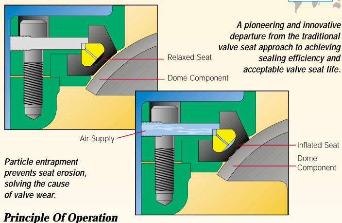
The Dome component closes beneath the seat(seal) when the seal is relaxed (not inflated), allowing a controlled gap between the seat (seal) and the closing member (Dome). Material is allowed to pass through or enter the controlled gap if, due to its characteristics, it is pulled into the gap by the action of the Dome component moving to its closed position.
